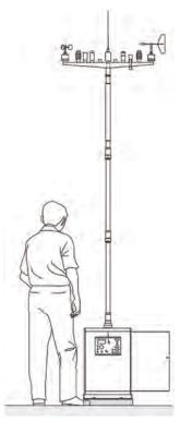
This sensor consists of a light wind vane pivoted on top of a housing. Inside the housing a compass is magnetically coupled to the vane. The sensor can be mounted directly on the sensor arm of the Automatic Weather Station 2700, Data Bouy 4700, or on different types of sensor brackets from Aanderaa and on a 25 mm O.D. vertical aluminum tube. When installed on brackets or tubes, the sensor must then be connected to the SmartGuard Datalogger or display unit by a separate cable.
