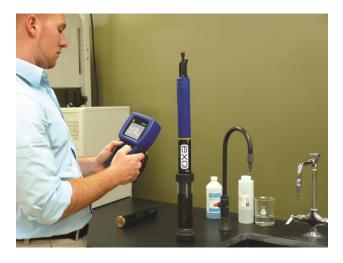
EXO1 and EXO2 sondes communicate wirelessly to an EXO handheld or computer for a safe, tangle-free calibration process
